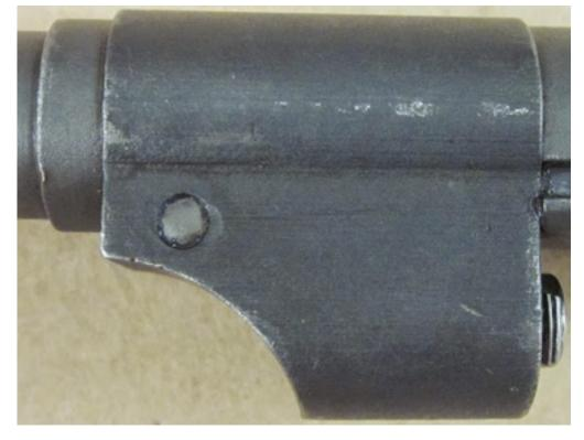
fitted with the common "swaged on" gas cylinder. Does anyone else have one of these early carbines?
